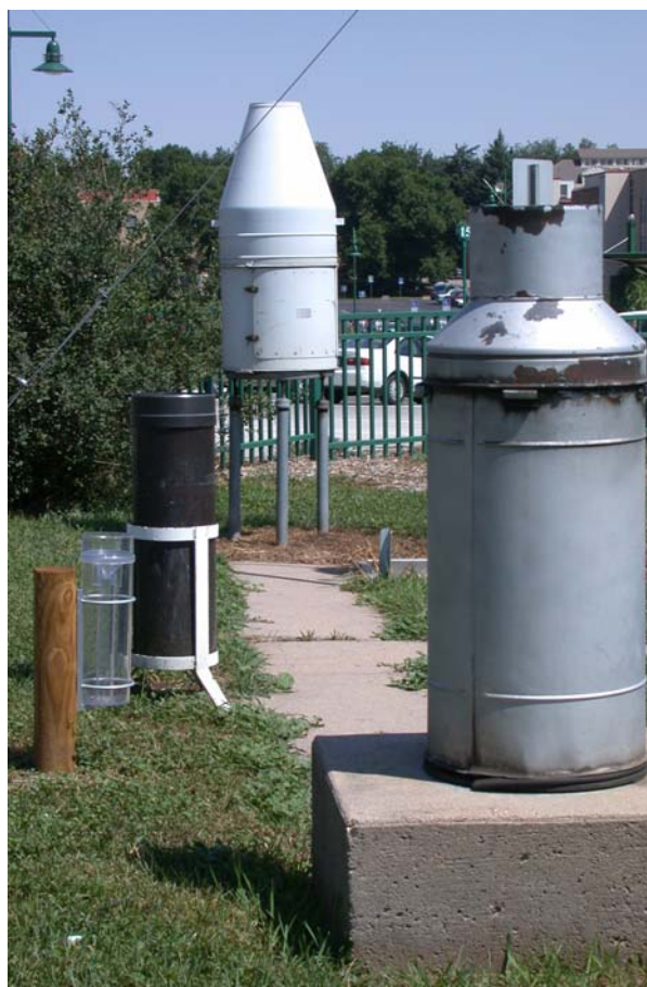
Figure 1. Example rain gauges at the Fort Collins, Colorado, National Weather Service Historical Climate Network weather station 05-3005-4.
