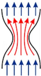
eighteenth-century Swiss scientist, who discovered that as the velocity of a fluid increases, its pressure decreases. Bernoulli's principle can be seen easiest through the use of a venturi tube (see left figure). A venturi tube is simply a tube which is narrower in the middle than it is on the ends. When the fluid passing through the tube reaches the narrow part, it speeds up. According to Bernoulli's principle, it then should exert less pressure.
