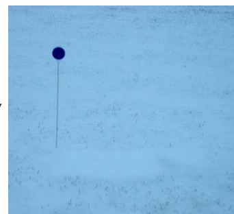
Without something to mark the location of the board, you can easily lose it after an inch or two of snow.
