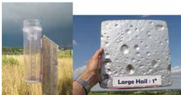
Figure 1. CoCoRaHS Rain Gauge and Hail Pad
